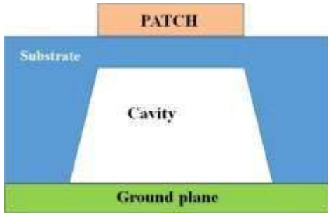
Figure 2. Micro-Machined Patch Antenna
