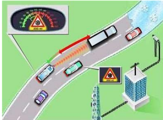
Fig. 1. Intelligent infrastructure and intelligent vehicles to warn about slippery road ahead.
