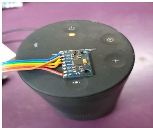
Fig. 3: IMU unit mounted on a vibrator.
